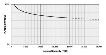
**Figure 3.** Specific propulsion power (at any constant speed)
