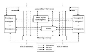
**Figure 1.** Three flows in a typical container shipping system
