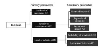
Figure 2. Improved parameter structure based on FMEA for container shipping operational risks
